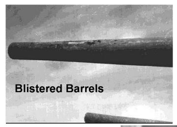
Between the 11 min ordeal, and some of the battles from ship to shore, the projectiles burned the paint off the gun barrels.(see photo).
